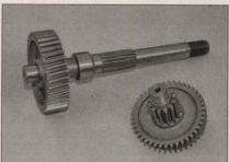
7.32 Check for damage to the pinion teeth and shafts
