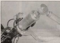
5.11b Hold the adjuster nut and tighten the locknut with the special tool
