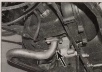
14.6a Exhaust downpipe is located on the underside of the scooter
