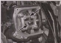
28.4 Check the rocker arms (arrowed) for clearance at TDC
