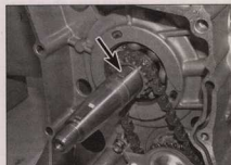
18.8 Location of the starter clutch Woodruff key
