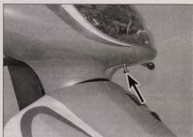
29.2a Headlight adjuster screw (arrowed) located underneath the light unit
