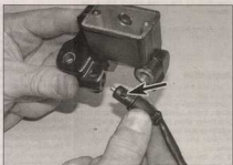
5.10 Remove the brake light switch. Note the retaining tab (arrowed)
