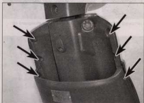
8.13a Front panel fixings (arrowed) in the kick panel ...
