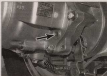
25.3 Gearbox oil should be level with the lower threads (arrowed)
