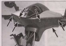
8.7a Check for screws (arrowed) along the outside edges
