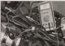
3.5b HT coil primary winding check
