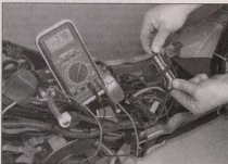
3.6 HT coil secondary winding check
