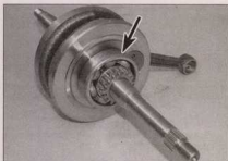
21.6 Check the main bearings on both sides of the crankshaft
