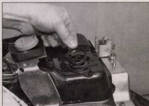
11.4d Note the location of the seal
