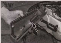
3.8 Check the air intake duct (arrowed) for obstructions
