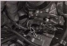
7.11a Detach the outer cable from the bracket (arrowed)
