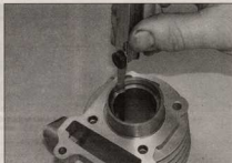
15.2 Measuring the installed piston ring end gap
