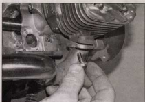
14.6b Downpipe fixings may require spraying with penetrating oil
