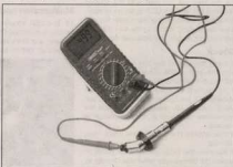
3.8 Measuring the resistance of the spark plug cap
