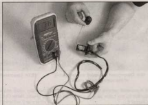
11.6 Set-up for testing the fuel level sensor
