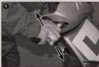
Hold the front brake on and pump the front suspension up and down to check operation
