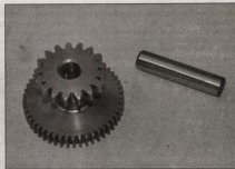
18.9 Inspect the idler gear and shaft for wear
