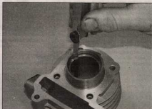
15.2 Measuring the installed piston ring end gap
