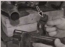
10.3d Note the location of the damper (arrowed)
