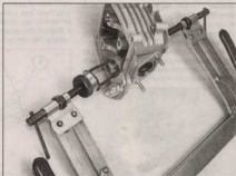
12.3a Compress the valve spring carefully...
