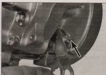
12.2 Location of the brake arm clamp bolt (arrowed)
