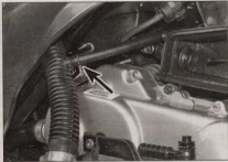
3.9 Inspect the hose union (arrowed) and clip
