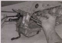
20.29 Installing the camchain tensioner blade
