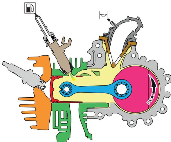
When the engine is running, fuel is injected directly into the combustion chamber.
