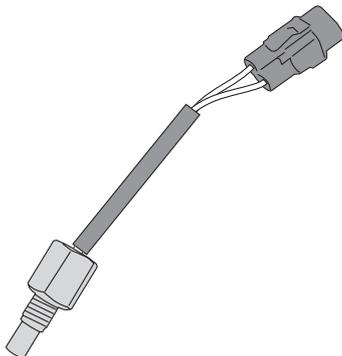
Located on the cylinder head, this sensor informs the ECU of the engine's thermal state. The ECU will modify the opening time of the injector based on the data sent by the temperature sensor.
