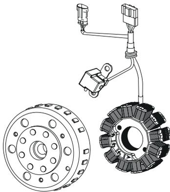
The current generator supplies electricity to the vehicle and recharges its battery. It delivers alternating current which is transformed to direct current by the voltage regulator.
