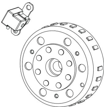
Pulse wheel fixed to the magneto flywheel.
