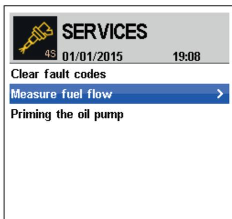
The flow measurement for the fuel pump must be carried out using the TEP2010 tool (Service functions).
