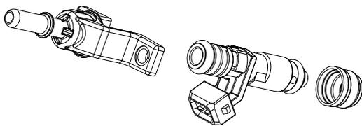
The fuel injector, controlled by the computer, injects the fuel required to run the engine.
