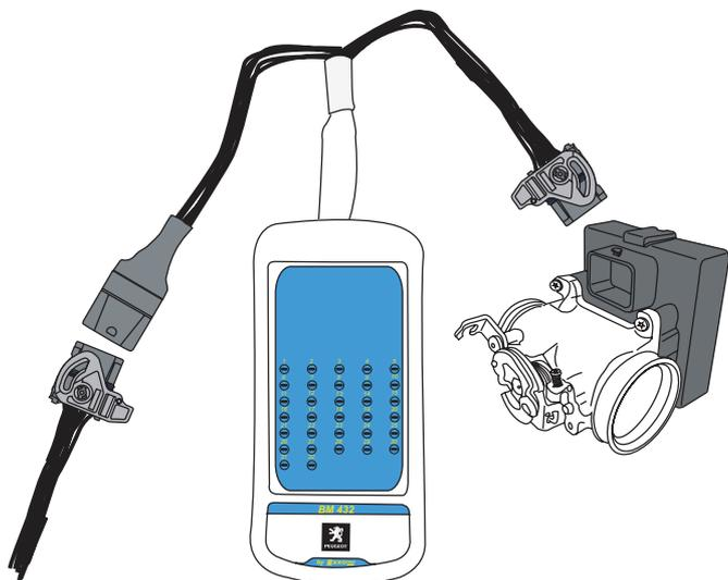
The new wiring harness feature sealed connectors. These connectors no longer allow you to carry out electric checks that are necessary for diagnosing the system.
