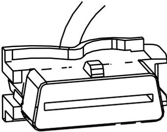
The OBD connector allows you to connect an approved diagnostic tool and check the injection ECU using standardized queries on the vehicle's compliance or the presence of anomalies.
