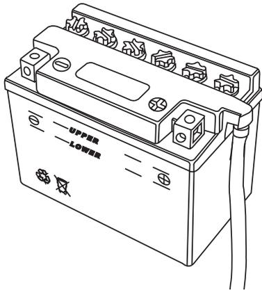
The battery is essential for the operation of the system. The minimum battery voltage necessary for the ECU to function is 8.5 volts.
