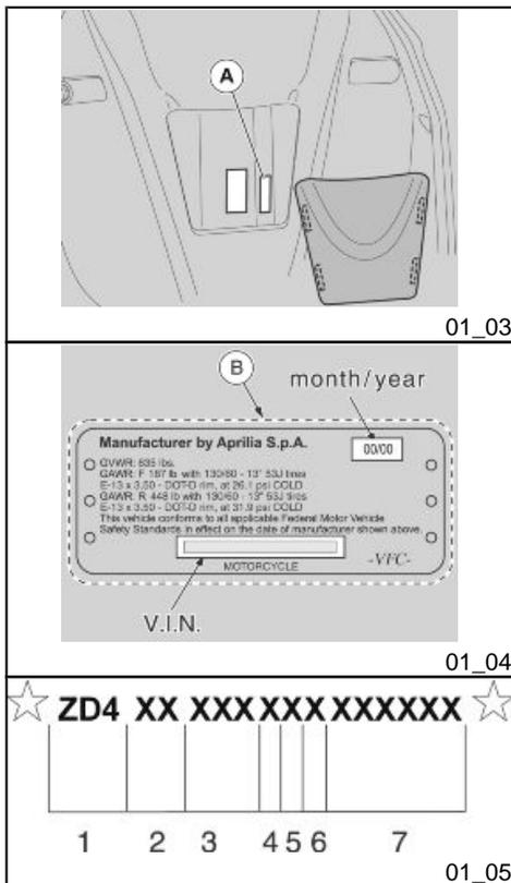
Description of the vehicle identification number (V.I.N.) stamped on the chassis headstock «A».
